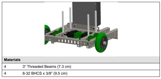
3 Attach the battery shelf to the threaded beams as shown below and tighten the mounting screws.
